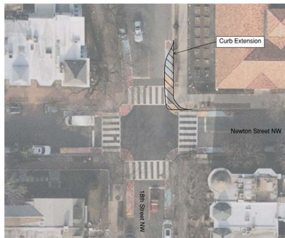
Figure 1 – Proposed curb extension at northeast corner of 18 th St & Newton St NW
