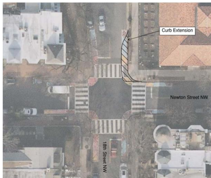
Figure 1 – Proposed curb extension at northeast corner of 18 th St & Newton St NW
